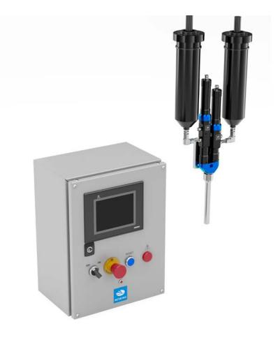
The LiquidFlow 2 is a versatile and efficient metering and mixing system for accurate dispensing of small beads and shots of two-part materials. One of the major benefits with this machine is the DC electric drive unit and progressive cavity pump technology which ensures very precise dispensing with high economic efficiency at the same time. Due to the compact size of
