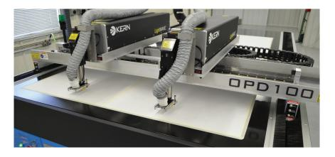
The OptiDual system is equipped with dual laser sources instantly doubling your laser cutting production. The KCAM laser software controls each laser independently allowing both lasers to be tuned to equal power. This feature ensures consistent cutting results from both lasers over the entire work area. The second laser can be disabled allowing full range of table motion for the master laser.
