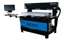
model and the Y axis is a moving table that increases the accuracy and speed while cutting. Like all Kern systems the MICRO is a turnkey package including the computer, software and downdraft vacuum system.
